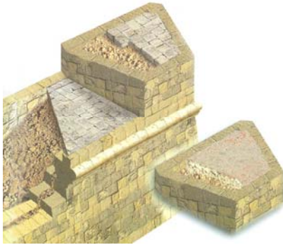
Figure 10. Graphic reconstruction of the construction of a Parapet and Embrasure (Courtesy: Stephen Spiteri)
